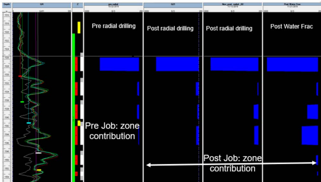
Figure 17—Time-lapse Injection Logging Shows improvement in conformance particularly after High rate flushing Operation post RJD Treatment
