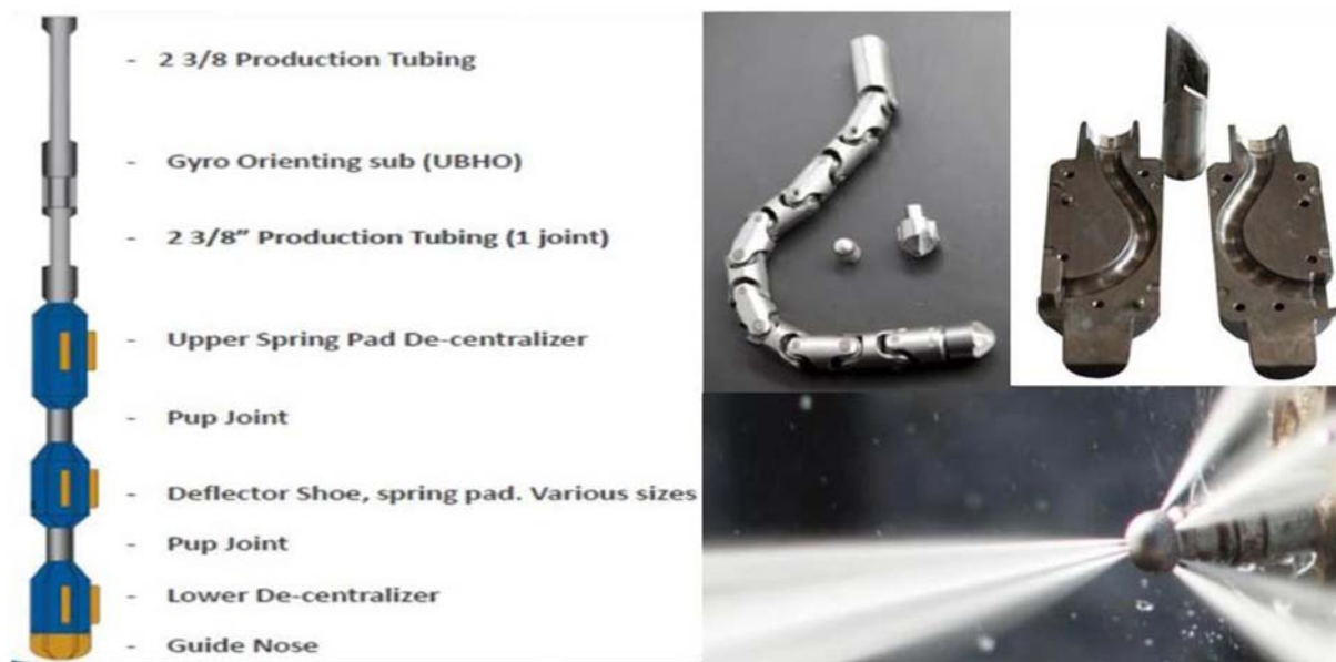
Figure 2—Typical Deflector Shoe BHA for RJD Operation (left), Cut section of Deflector show & Picture demonstrating Flexibility of Flexshat (Top Right) & Close up of Jetting Nozzle (Bottom right)
