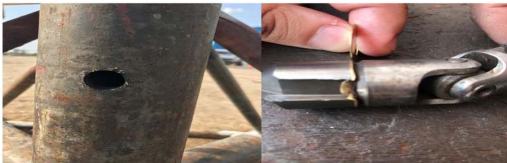
Figure 11—Milled 1.5' window post milling function test (a) and broken confirmation ring (b)
