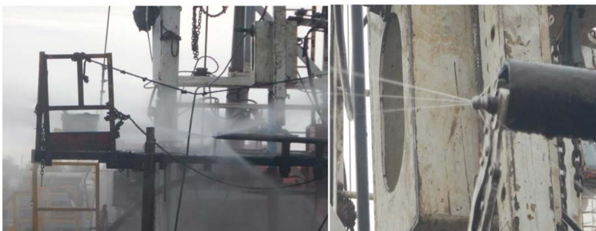
Figure 14—Actual Function test of Jetting at High (left) pressure & Low(right) pressure
